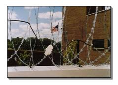
The SL-3 sensor is supplied, tested and pre-assembled in 3.0-meter intervals. Installation of the SL-3 Multidirectional sensor cable is very fast and simple; it is ready to mount into any new or existing
